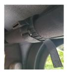
Undo Velcro and place clip over roll bar (both sides) slightly angled down Re-thread Velcro back thru ring and leave slightly loose
