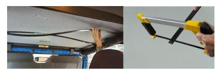
Pushing on Bow near one end flex Bow upward (Bow should "snap" in place)
