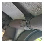
Once bow is in place tighten Velcro straps on both ends
