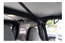
Insert Bow in both ends of clip and leave hanging downward
